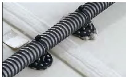
**PMB5 mounts** are fixed in position with paste-like industrial glues and are outstandingly well suited for the secure fastening of lines to locations that cannot be drilled, for example to attach sensor cables for monitoring the operating condition.
