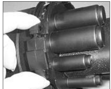
42. Secure the cover to the base using the snapperband.
