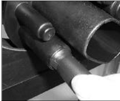
20. Pull the Cablelok until the flange "snaps" into place.
