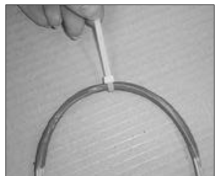
18. Fit a cable tie to the unit tubes at position 'C'.
