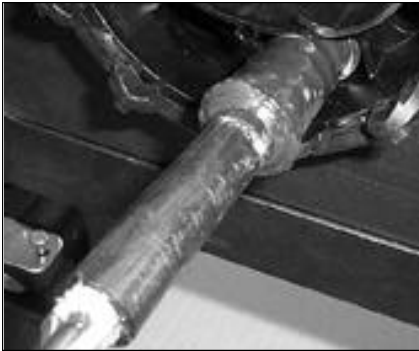
19. Push the Cablelok back into the port.
