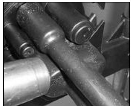
69. Recover the heatshrink on to the cable.
