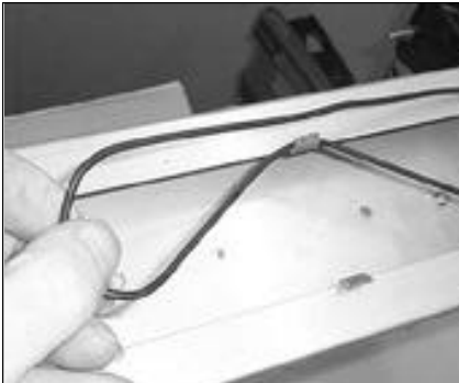
19. Remove the loop restraining strap on the basket.
