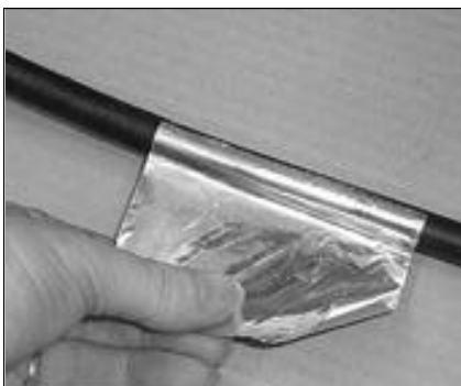
13. Apply the foil adjacent to the abraded area at position 'A'.
