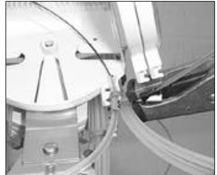
30. Tighten cable ties using a suitable tool.
