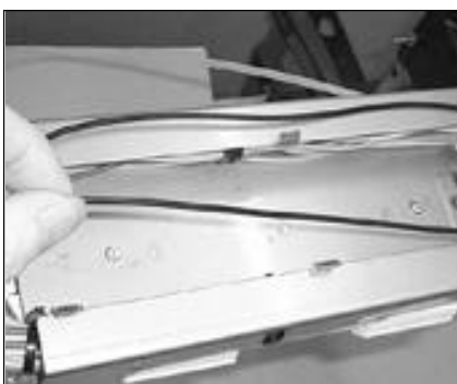
70. Remove the loop-restraining strap on to the basket.
