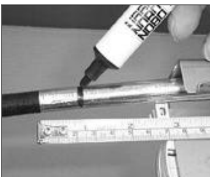
25. Mark the foil 20mm from position 'A'.
