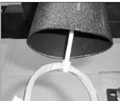
22. At position 'C' bend fibre tubes and insert in to the oval port, with the aid of the cable tie.
