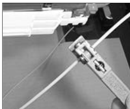
62. Cut the loose tube at the 70mm mark, ensuring not to damage the fibres.
