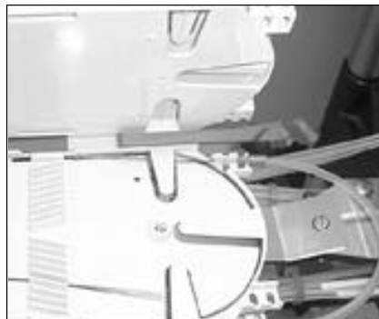
32. Fit the tray holder at the opposite end of the tray.
