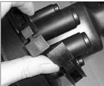
43. Release the snapperband and remove the cover.
