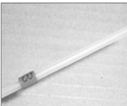
61. Place the correct number of coloured markers provided, onto each of the flexible tubes.
