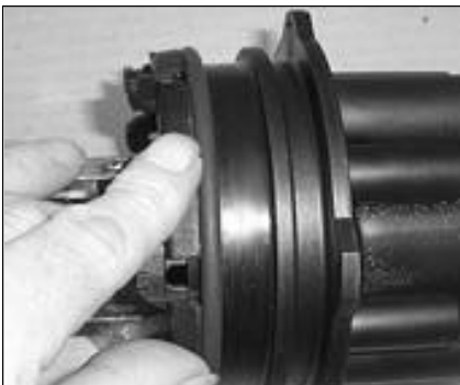
40. Ensure the 'O' ring is located in the position shown.
