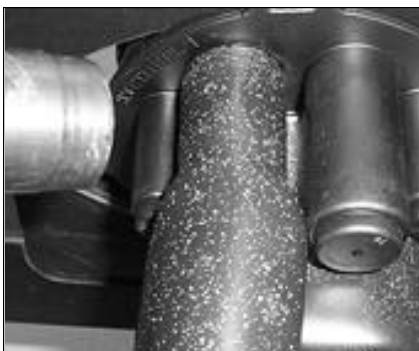
49. Place heatshrink on to port and recover, leaving approximately 10mm unrecovered at the end of the port.
