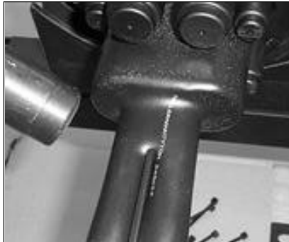
38. Recover the heatshrink onto the cable.
