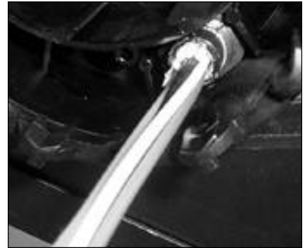
21. Holding the Cablelok adjust the cables. The cable sheath should protrude 5 to 10mm up from the Cablelok.
