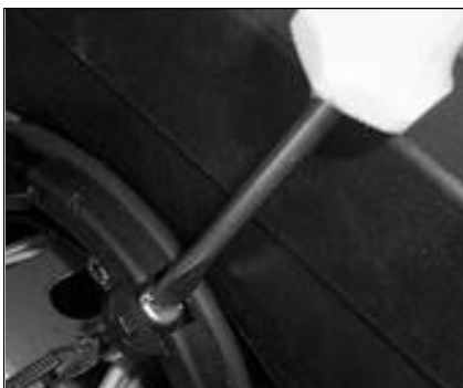
67. Secure the central strength member using the fixings provided. Refer to steps 28 to 30 for details.
