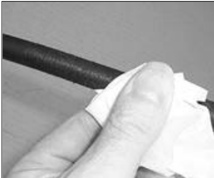
64. Clean the abraded area of the cable using an IPA wipe.
