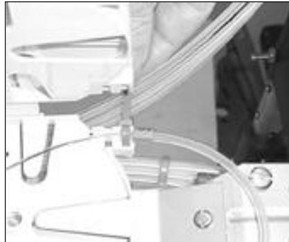
29. Fit the flexible tube to the tray and use cable ties to hold in position.
