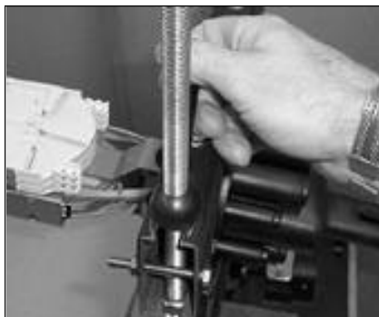
44. Fit the closure into the installation bracket, for easier installation.
