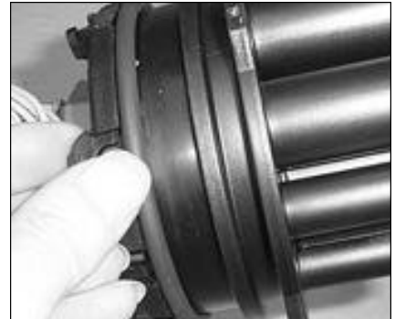
39. Ensure the 'O' ring is located in the position shown.
